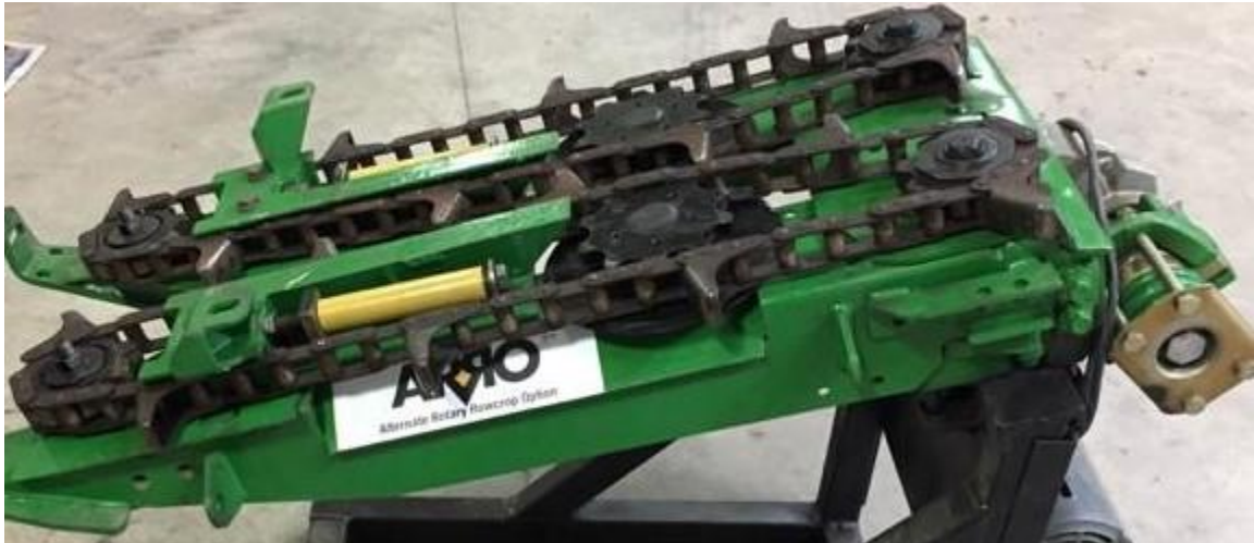
ARRO – Alternate Rotary Rowcrop Option conversion kit on a John Deere corn head unit
